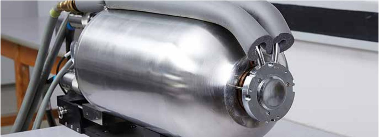
Neutronengenerator am Fraunhofer INT
